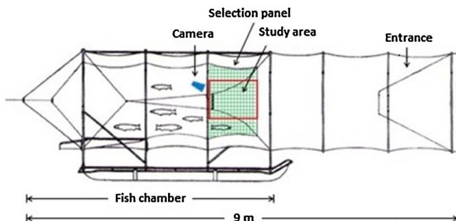
**Fig. 3.** The northern side of the experimental pontoon fish chamber with 50 mm square mesh selection panel, showing the placement of one camera and corresponding study area. The set-up was identical on the southern side.
