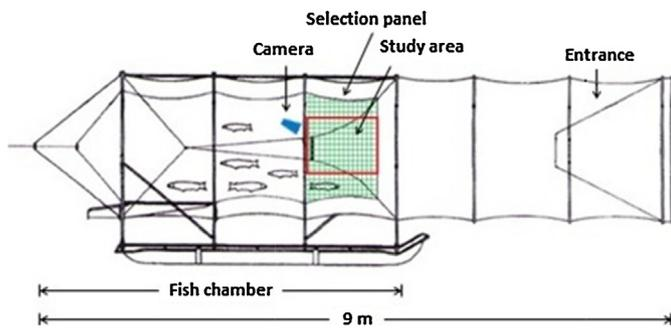
**Fig. 3.** The northern side of the experimental pontoon fish chamber with 50 mm square mesh selection panel, showing the placement of one camera and corresponding study area. The set-up was identical on the southern side.
